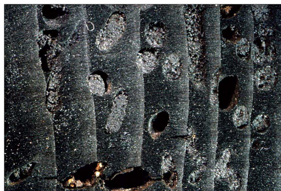
Figure 5. Insect galleries, partially with faecal pellets from larvae.
